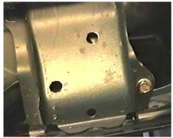
14. While baseplate is still attached to metal bumper, drill remaining holes with the 13/32" drill bit. Using baseplate as a template, drill 1 1/4" hole in the side of metal bumper, refer to photo in step 7 for location.
