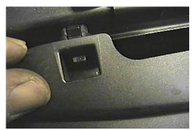
1. Insert small flat screw driver into clips to release all four, remove grill, and set aside.
