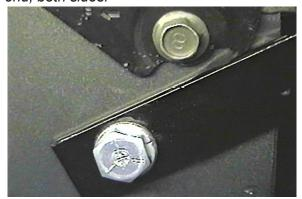
11. 2002-03 Models: Align support brace with existing hole. Hole may need to be drill out with the 13/32" drill bit. Insert item 3 into drilled 1 1/4" hole to align with 13/32" hole, items 5 and 6, and tighten. Be sure and use loctite on all bolts before tightening. Go to step 14.
