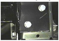
15. Using the 1 1/4" hole saw, drill hole in the side of metal bumper. Refer to photo in step 7 for hole location. Insert item 3 into 1 1/4" hole and fasten to items 5 and 6 for the two front holes and lower side hole, both sides. Tighten all bolts. Be sure and use loctite on all bolt before tightening.
