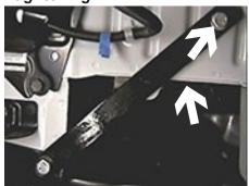
12. 2004 Models: Drill out existing hole with the 13/32" drill bit if needed, on frame rail. Insert item 4 into opening on bottom of frame to align with drilled hole, items 5, 6 and 8. Be sure and use loctite on all bolts before tightening.
