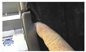
**4.** Remove phillips head push pin just forward of front tire and one inside wheel well on fascia.
