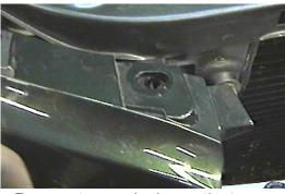
2. Remove two push pins on the top, one just behind, pull forward, and set aside outer grill supports. On top side of fascia are 5 push pins to be removed.
