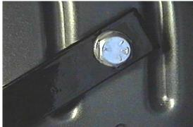
10. 2002-03 Models: Drill out existing hole with the 13/32" drill bit, on frame rail. Insert item 3 into frame end to align with drilled hole, items 5, 6 and 8. Be sure and use loctite on all bolts before tightening.
