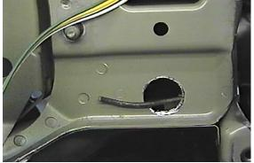
9. 2002-03 Models: Using the 1 1/4" hole saw, cut hole into lower chamber of frame end, both sides.
