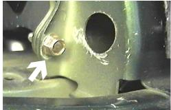
7. 2002-03 Models: With the 14MM socket remove the two outer bolts from the metal bumper, both sides. 2004 Models: Replace factory metric bolt with 8MM-1.25 x 30MM Hex Bolt.
